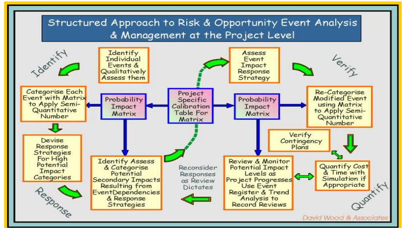
Figure 1: Structured semi-quantitative scheme for identifying assessing and formulating response strategies to individual identified events.
